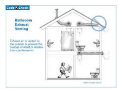
intermittent ventilation or 20 cubic feet per II minute for continuous ventilation. Ventilation air from the space shall be exhausted directly to the outside.
